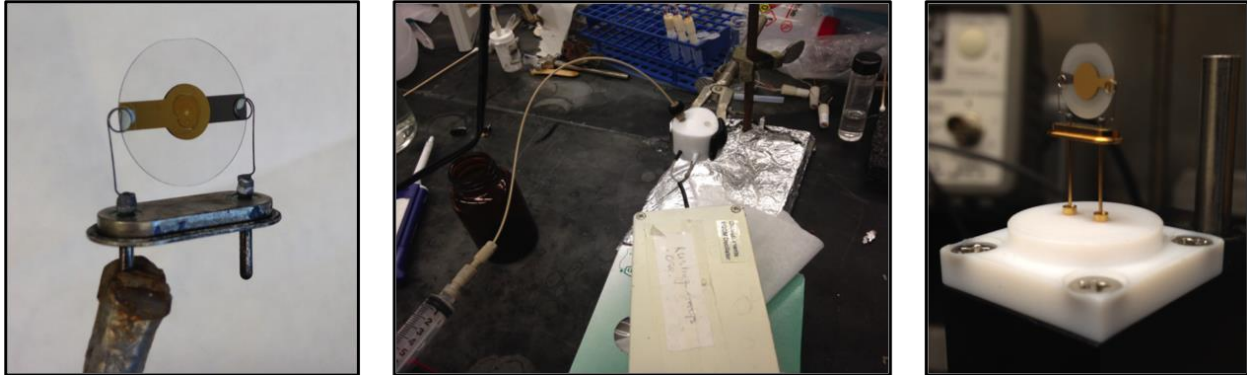
Figure 11. (left) A QCM resonator coated in a Cell-Tak™ film. (center) An EQCM equipped with a flow-cell and syringe pump in which real-time protein film mass can be monitored as a function of flow-rate. (right) A static QCM resonator used in conventional QCM analyses.
